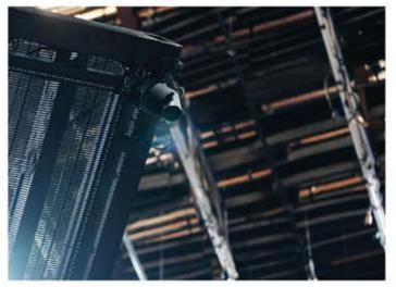
Cube v3 glows with custom visual effects designed by deadmau5. The cube can spin 360 degrees and dip 45 degrees during performances. The system uses a real-time IP network to communicate with the PTZOptics cameras over Artnet. The cameras can then position themselves remotely to match the movement of this massive cube and keep the images straight.
