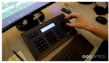
The PTZOptics Producer Kit comes with a HuddleCamHD Joystick serial controller. They used the device to set camera presets of each podium, the choir, and wide shots. This is optimal for volunteers to easily adapt to controlling the cameras, simply by recalling presets made by the technical
